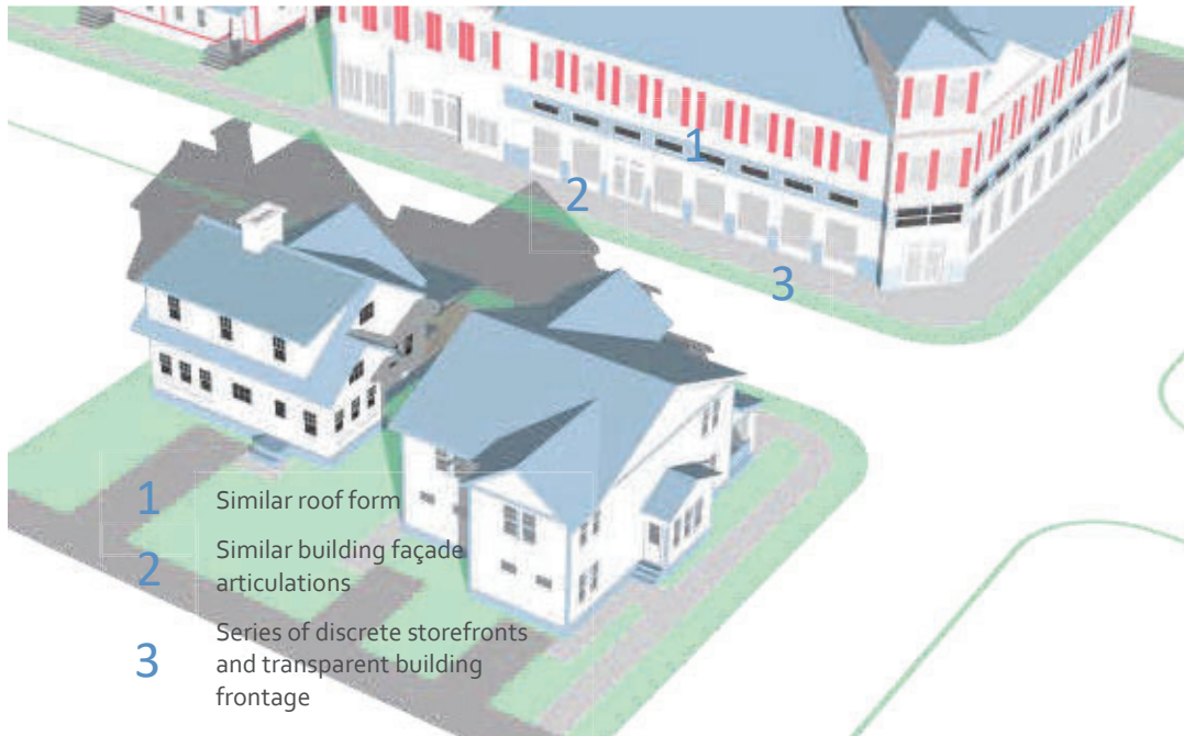
Figure 5.8.C(3): Appropriate Building Form
