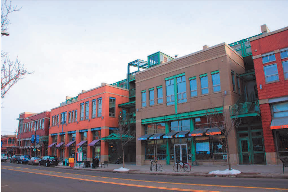
Figure 5.7.E(3)a: Example of Front Façade Offsets
